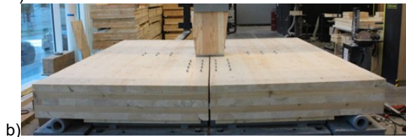
Fig 2: Self-tapping screw shear reinforcement pattern schematic (a); exemplary photo (b).
