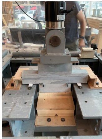
Fig. 5. Test setup and instrumentation for the UHPFRC.
