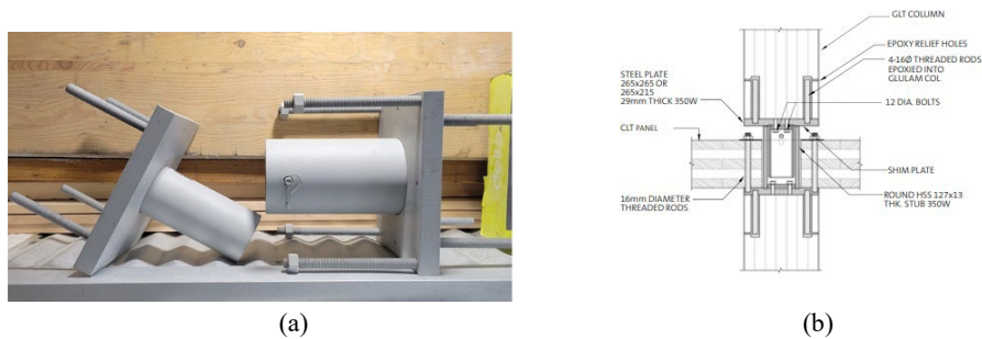
Fig. 1. Steel HCS connection for timber structures, (a) dismantled connection, and (b) A schematic sketch of the steel HSS connection joining CLT panels and Glulam columns (photos courtesy of Fast + Epp).
